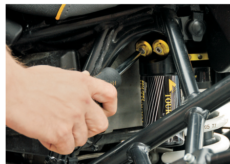
The compression in the high and low speed range can be adjusted on shock absorbers with a piggyback reservoir.
