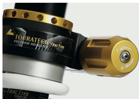
From the "Level 2" version onwards, Travel series shock absorbers have a hydraulic spring preload.
