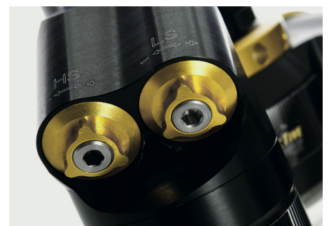
Travel "High End" and Travel "Extreme" series shock absorbers provide adjustment options for compression damping.
