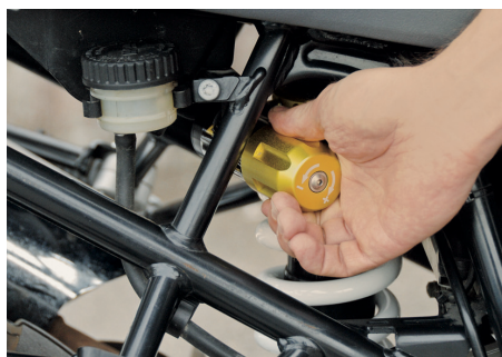
The preload of the spring adjusts the balance of the motorcycle.
