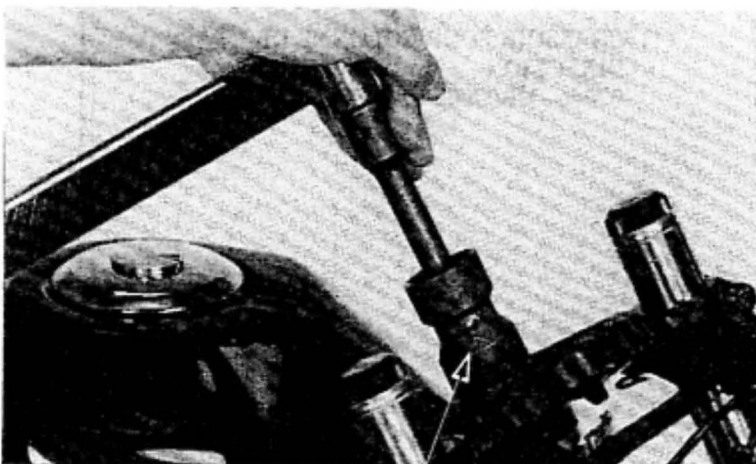
(1) LOCK NUT WRENCH, 30 x 32 mm 07716-0020400 EXTENSION BAR 07716-0020500
