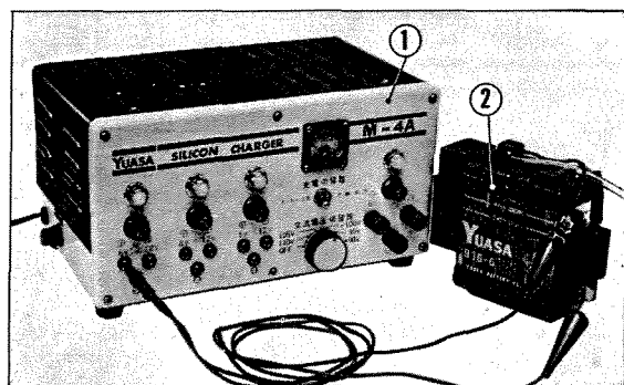
Fig. 5-18A. ① Charger ② Battery
